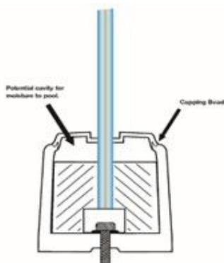
*Note : Balustrade channel designs with a top cap or bead may create a potential internal cavity for water to pool. Also, where dry glazed systems are used, consideration must still be given to ensure that any water which enters the channel is able to drain away.*
